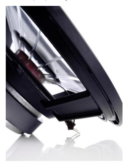
The modeling software was applied to optimize the curvature parameters of the clear X3P hyperboloid, and so obtain the lowest mass and highest rigidity. Furthermore, the software optimized the spoke-like mechanical reinforcements on the back surface, where 15 slender spokes of X3P material taper gradually from the central hub up to the outer rim with a slightly steeper hyperbolic curvature, for the ultimate pistonic behavior.
