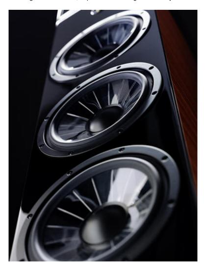
For over a decade, VA has applied Spider-Cone<sup>™</sup> technology to the bass drivers of its larger loudspeakers. The technique braces each cone with a spoke-like pattern of X3P ribs molded onto the back. Spokes increase cone rigidity while limiting mass, and result in superior damping of the driver.
